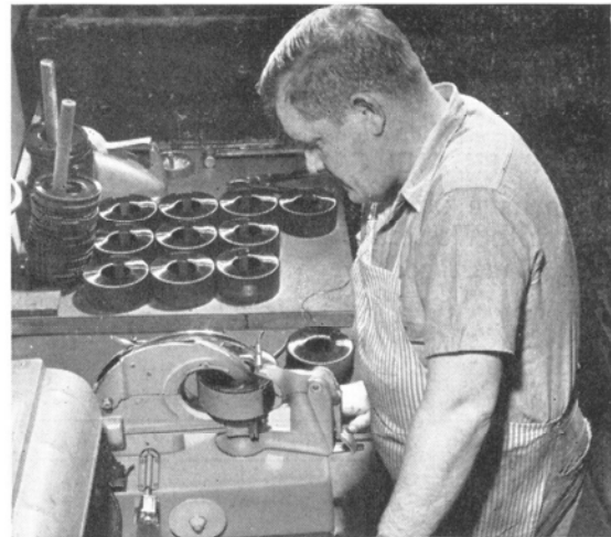
The coils for Variac ® autotransformers are wound on the GR-designed machine, shown above, which applies an evenly spaced winding, accurately banked.
