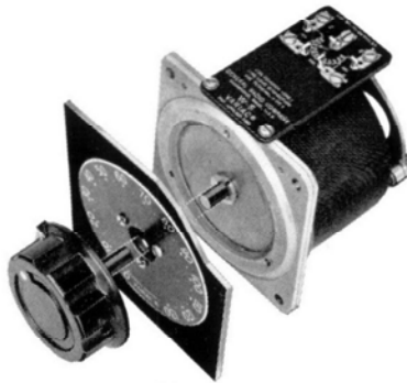
Types W5, W5H Uncased Model. Mounting Base: 4½ inches square. Depth Behind Panel: 4 inches. Four Mounting Holes on ¾ inch square. Max. Panel: ⅜ inch.
