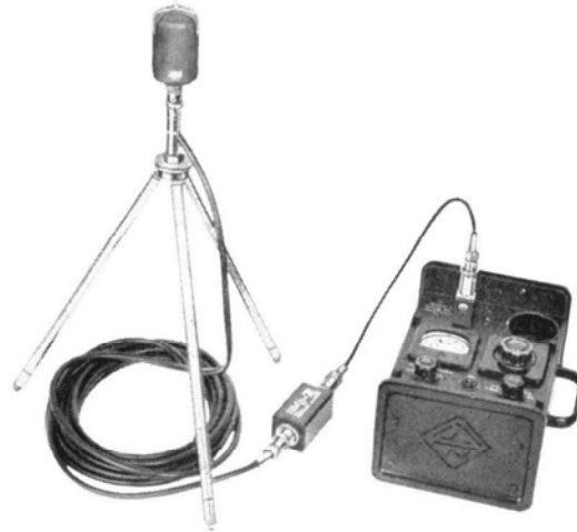
(B) Microphone and transformer plug into the sound-level meter as shown above.
