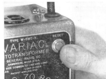
Overload protector, a new feature on portable models, is reset from front panel.
