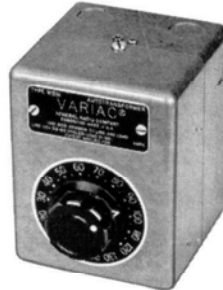
Type W2M Cased Model, with Conduit Knockouts. Case Dimensions: Width 4 1 / 8 in., Height: 5 9 / 16 in., Depth: 4¼ in.
